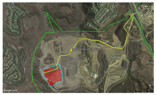
Green line: Cyan line: Red polygon: Prima Deshecha Landfill approximate boundary Capistrano Greenery Composting Operation approximate boundary Area sources representing receiving area, composting/curing piles, and screening/storage/loadout area Representative on-site trucking route
